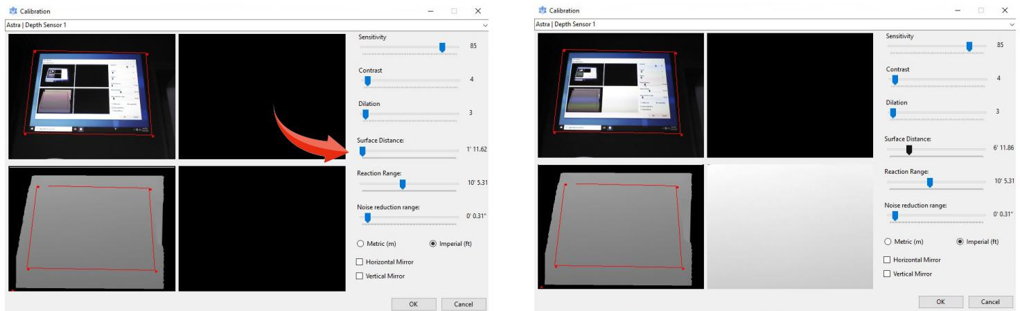
5. Slide the Reaction Range tab to the left, the lower right screen will turn black. Slowly move the tab to the right, until the lower right screen turns white. If a small corner remains black, that is okay. The important thing is to have the projected area entirely white.
