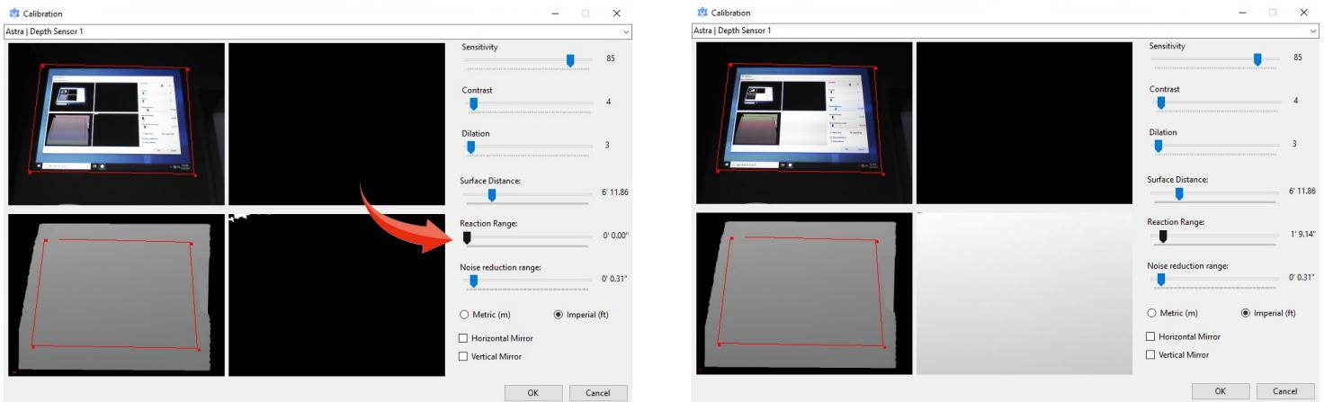
6. The Sensitivity, Contrast, and Dilation adjustments need never be touched and are preset at Sensitivity 85, Contrast 4, and Dilation 3.
