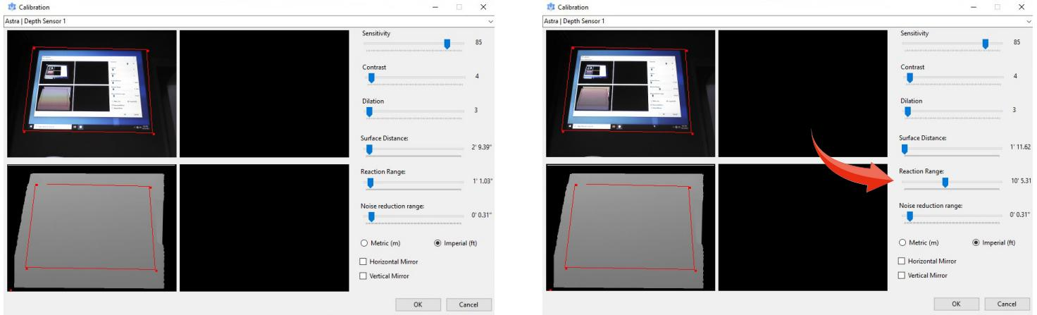
4. Slide the Surface Distance tab to the left, the lower right screen will turn black. Slowly move the tab to the right, until the lower right screen turns white, then stop. If a small corner remains black, that is okay. The important thing is to have the projected area entirely white.
