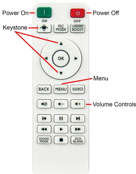
Once the projector is turned on with the Power On button and the system has warmed up, you may notice that the projection is not square. If this is the case, simply point the remote at the FX unit and press the Keystone button followed by the Up or Down arrows.
