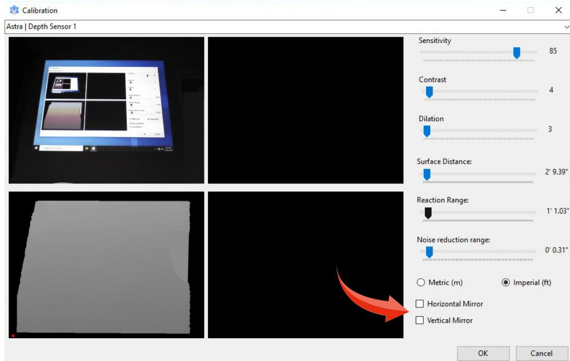
2. In the upper left window, use the mousepad to form a box around the projection. This will be done by left-clicking outside each corner of the image. When complete, there should be a red-lined box around the projected image. The box can be larger than the image, but not smaller.
