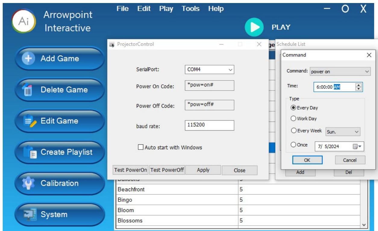
3. In the Projector Control window check the box next to **Auto start with windows**, click **Apply**, then minimize the window, **do not click Close**. The **Close** option shuts off the projector control panel, preventing the schedule from running.
