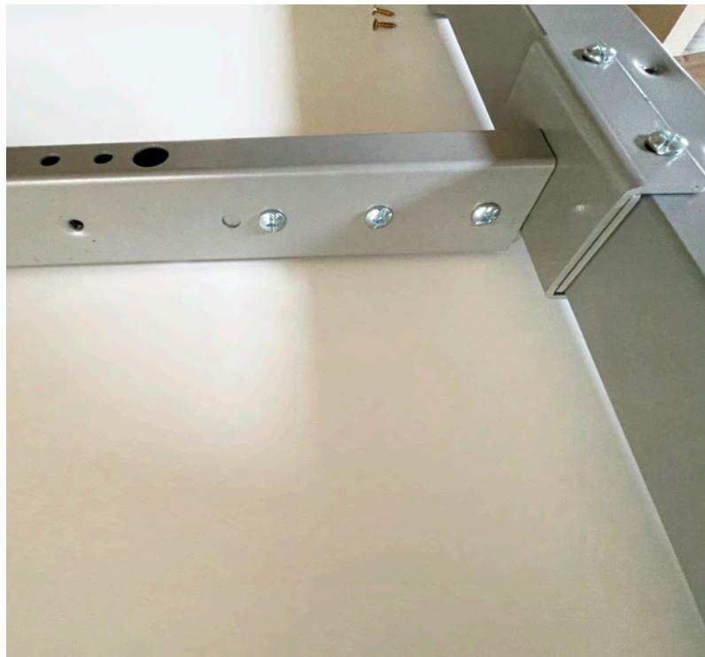
5. Attach a metal mounting flange to each of the center support beams, using the bevel head screws. Tighten firmly and insert it flange side down, into each end of the supports.
